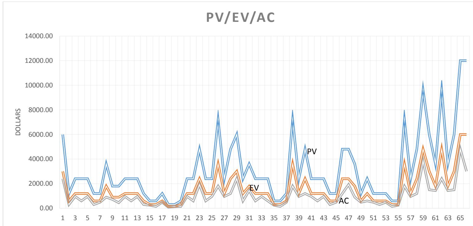
The Critical Ratio can also be used with earned values, bearing in mind that “progress” in earned value nomenclature is expressed in monetary units, and we have only three measures instead of four, actual progress is EV, scheduled progress is EV and Actual Cost is AC.
