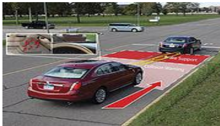
Figure 14 Ford's Collision Warning with Brake Support System [21]
